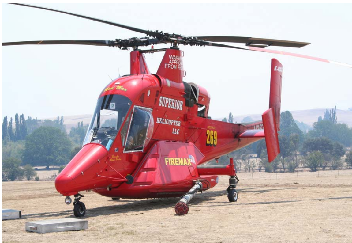
Helitack 269, a Kaman Kmax Type 2 firebombing helicopter, part of the national aerial firefighting resource.
