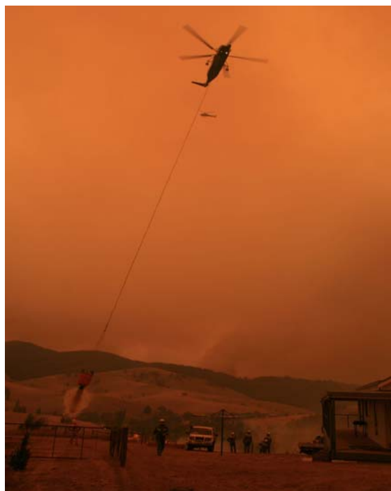
Helitack 348, a Sikorsky 61N with 3,400lt bucket
