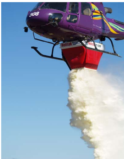
Helitack FT2100B3 delivery system
